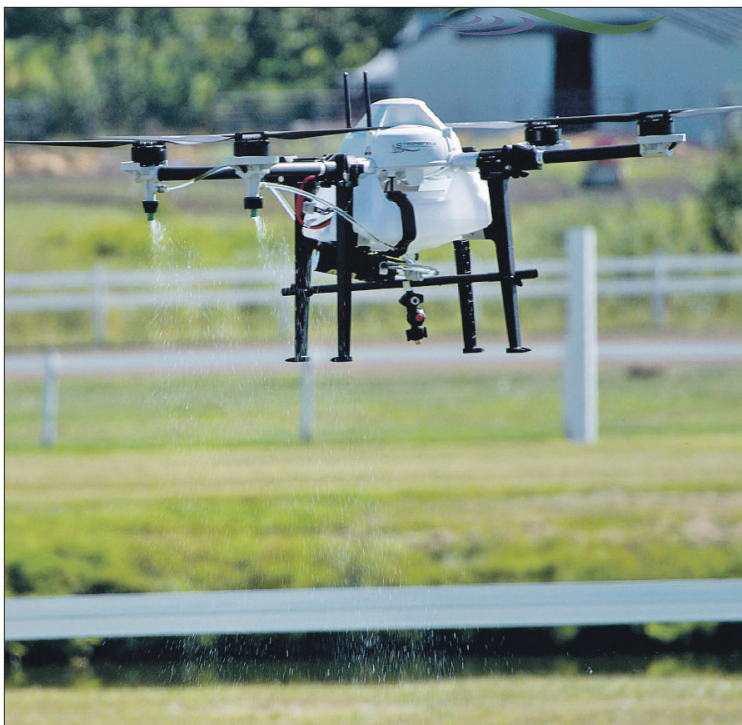
This Strongfield Environmental Solutions drone uses course nozzles that emit large droplets, which are less likely to drift off target compared to fine droplets that spraying drones usually use.
