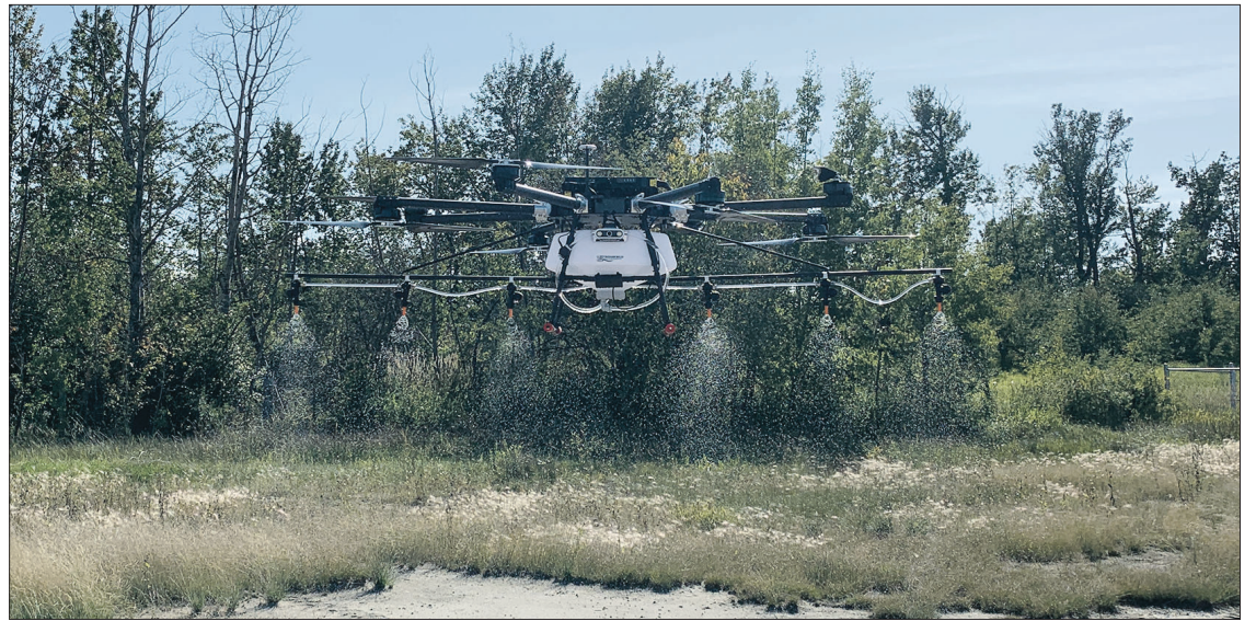
Drones are commonly used to spray crop protection products in Asian countries such as South Korea and China. However, little is known about how effectively drone sprayers hit their target compared to spray planes and helicopters.
